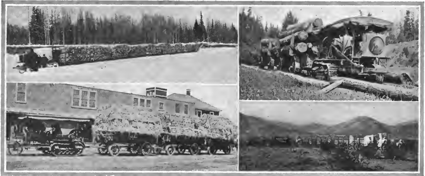
Upper left—Caterpillar tractor hauling fifty-two cords of timber at Fairbanks, Alaska. Right—Caterpillar used in logging. Lower left—Hauling hay in California. Right—Use in hauling equipment and material for a water development in Los Angeles, Cal.
